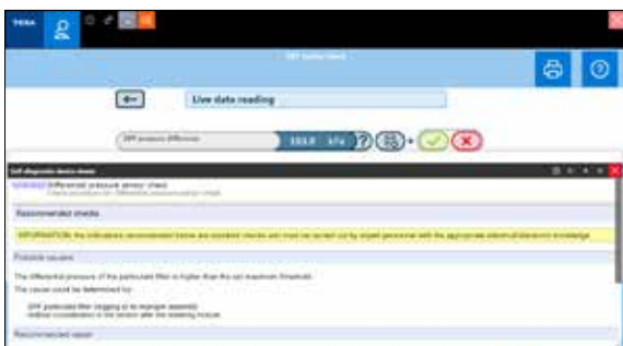
Error parameter reading with technical sheet
