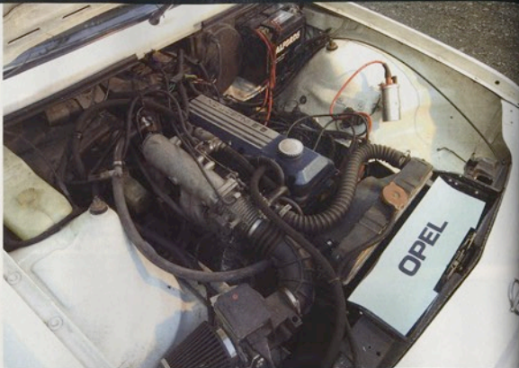
2.2-litre Carlton motor is an easy swap using the 2-litre gearbox.
