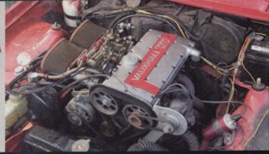
The mighty 16-valve XE drops into the bay a treat.
