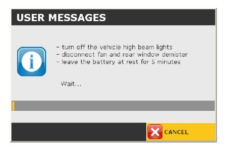
The test results could be unreliable if the battery is too low.
