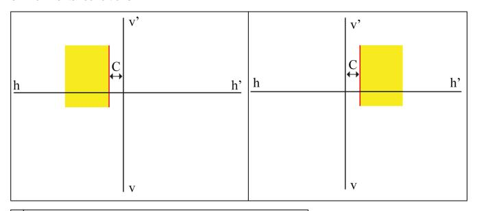
C Horizontal distance of the cut-off line from the central line.
