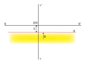
A Cut-off line. In the *Light Geometry* menu, set the nominal tilt indicated by the manufacturer.
