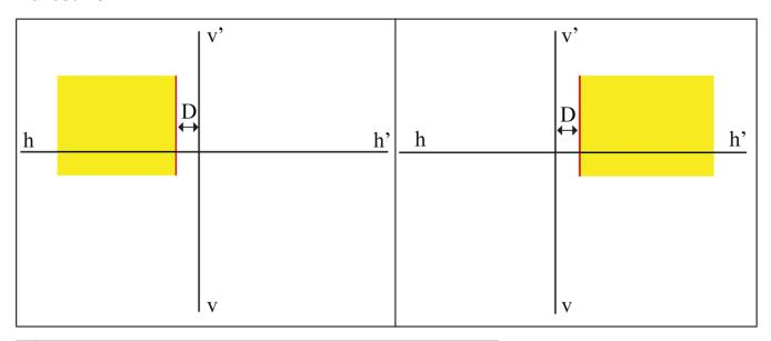
D Horizontal distance of the cut-off line from the central line.
