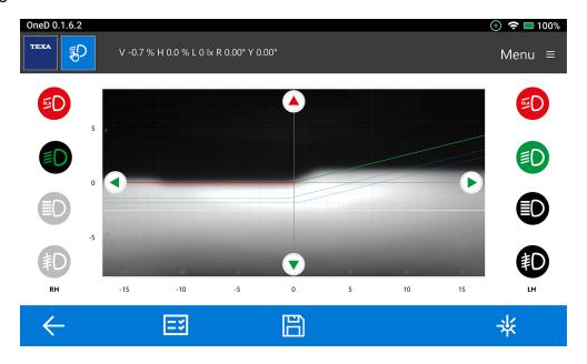
In the upper part of the screen, the test results are displayed in real time:
