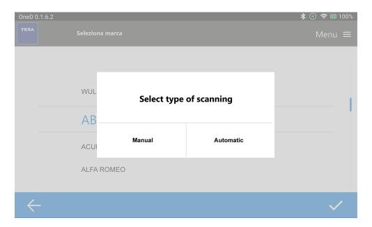
By pressing Automatic, the software automatically identifies the *Model Variant*.
