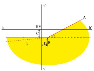
**Hotspot:** centre of the light beam in high beam  $\frac{h}{-}$  headlights.
