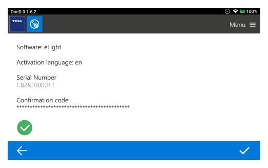
2. Enter the Confirmation code if the tool is not connected to an active Wi-Fi network.
