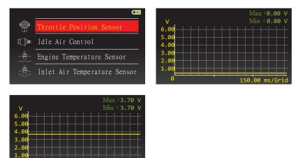
Enter Throttle Position Sensor and connect positive probe (Red) with sensor and the negative probe (Black) with chassis ground of the vehicle in order to perform measurement.
