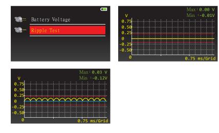
Enter Ripple Test and connect positive probe (Red) with sensor and the negative probe (Black) with chassis ground of the vehicle in order to perform measurement. X Attention: Ripple Test is only for measuring Ripple Test. Please DO NOT attempt to measure any other type of value under this setting.
