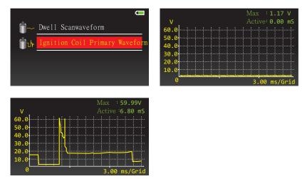
Enter Ignition Coil Primary and connect positive probe (Red) with sensor and the negative probe (Black) with chassis ground of the vehicle in order to perform measurement. Max. Voltage is out of range, press  $\blacktriangle \nabla$  to modify the range of Voltage measurement.
