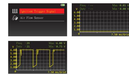
Enter Idle Ignition Trigger Signal and connect positive probe (Red) with sensor and the negative probe (Black) with chassis ground of the vehicle in order to perform measurement.
