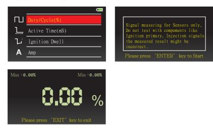
Enter Duty/Cycle (%) and connect positive probe (Red) with sensor and the negative probe (Black) with chassis ground of the vehicle in order to measure the percentage.
