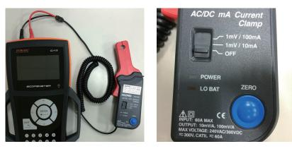
Please select proper condition for the Current clamp measurement, for example in order to measure 1mV=0.01A with CA15, move the switch to the 1mV/10mA on Current clamp.
