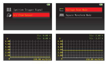
Enter Air Flow Sensor and connect positive probe (Red) with sensor and the negative probe (Black) with chassis ground of the vehicle in order to perform measurement. Analog air flow sensor is same as Voltage air flow sensor. Such as: Toyata Surf, Toyata Vios.
