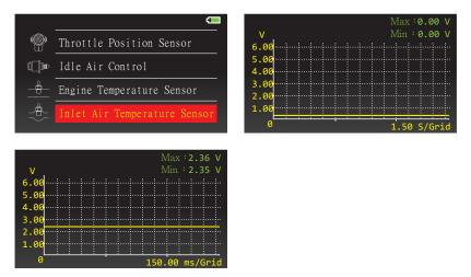
Enter Inlet Air Temperature Sensor and connect positive probe (Red) with sensor and the negative probe (Black) with chassis ground of the vehicle in order to perform measurement.
