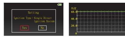
Enter Ignition System to measure RPM.
