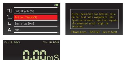
Enter Activation Time and connect positive probe (Red) with sensor and the negative probe (Black) with chassis ground of the vehicle in order to perform measurement.
