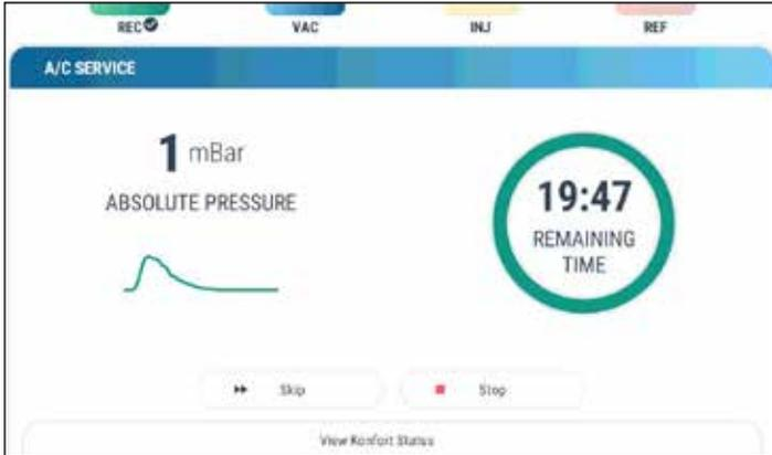
«Vacuum» phase: a vacuum is induced in the vehicle's A/C system to check for possible leaks.
