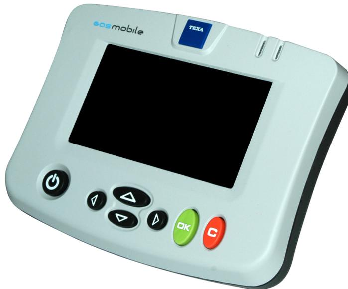
The **GAS MOBILE** software is contained within an SD CARD, (SD CARD specifically developed for the GAS MOBILE device) so that it may be quickly updated, even via Internet, to keep up with changes in norms or in order to add new functions.
