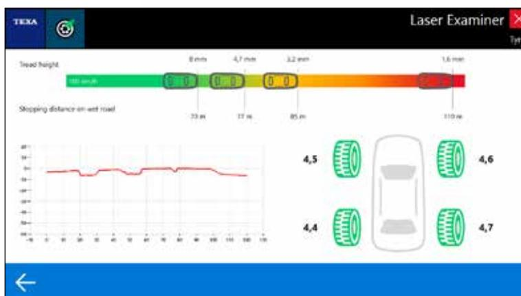
Tread measurement results with wear highlighted graphically.
